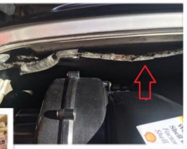
My father-in-law, Sid Cannon, and I agreed we needed to come up with something to tidy up that area, but replacing the pad with the engine in place was not really an option. To do that, the old pad would need to be removed, then the area prepped. Adhesive would need to be placed on the pad and the engine bay surface. The adhesive is pretty instant, and once the two
