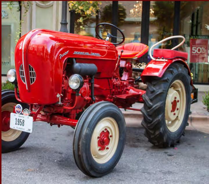
Our tractor had an 822-cc, single cylinder, air-cooled engine with Bosch fuel injection. It produced up to 14 HP to the rear wheels through a 6-speed transmission. It featured 3 power take-off shafts to power various implements. It had both front and rear hitches for trailers and implements.
