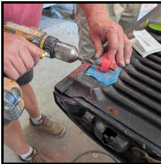
Sanding bushing to size
